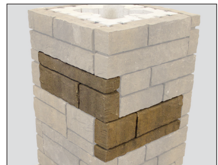
Diagram 25—Stagger veneers to break up lines
